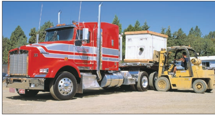
Complete pre-assembled valve vault ships with lift station.
